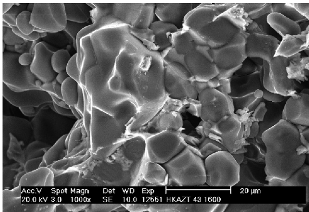
Fig. 4. Microstructure of the surface of Material AZT 1600, SEM micrograph, magnification 1000 \times .
